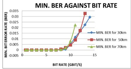
Fig. 7: The graph of Min. BER against Bit rate for 30km, 50km and 70km.
