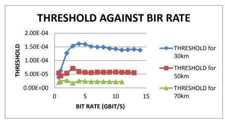
(iv). Graph of Threshold against Bit rate for 30km, 50km and 70km.
