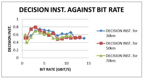
Fig. 9: The graph of Decision instant against Bit rate for 30km, 50km and 70km
